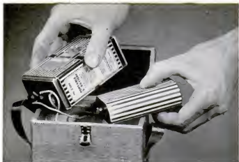
Two small batteries housed in the bottom of the cabinet form the tiny receiver's complete battery supply
